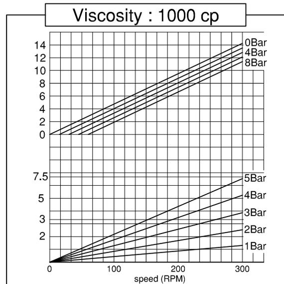
This data is based on very tough application. You can look the maximum power rate. And, when you selecting a pump, you must consider of kind conditions. For example, 'Temperature', 'Suction Conditions', 'Characters of Liquid'..etc
